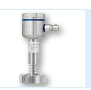
Application Diaphragm seals MD 50/51 with food law compliant screwed pipe connection for hygienic process separation of pressure measuring and control units in pipes or tanks. For mounting to Bourdon tube pressure gauges, pressure transducers and pressure switches. For installation in hygienic processes without dead spaces.
