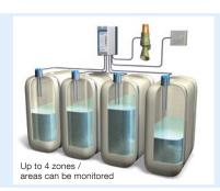
Application Suitable for use with electrically conductive liquids which do not foam excessively, are not viscous and not adhesive (bridging), e.g. water, emulsions or waste water. Ideal for generating alarms in large installations and facilities. Several zones (also large areas) can be monitored simultaneously with electrodes (probes) at various points.
