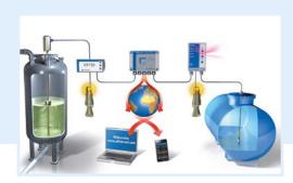
**Application** The event reporting system EMS 442 is ideal for a wide range of industrial remote monitoring tasks. Up to 4 analogue measured values and 4 digital limit values can be monitored with a single unit. In connection with the AFRISO Net web service, data can also be visualised, logged and managed.
