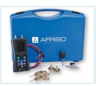
**Application** For differential pressure measurement and flow rate adjustment in heating and refrigerating systems during hydraulic balancing. To be used with VarioQ thermostat valves, VarioQ combination blocks or standard line fittings with measuring function (such as Gampper Vanitus Eco / Vanitus L). If VarioQ valves are used, hydraulic balancing can be done directly at the radiator. It is neither necessary to know the pipeline system nor to perform complex calculations.
