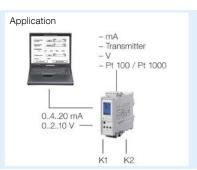
Description The digital multi-purpose transducers are freely programmable digital transducers with two analogue outputs and up to 4 relays. Current up to 20 mA (also bipolar), voltage up to 10 V (also bipolar) or a three-wire technology potentiometer are possible input signals. In addition, a supply for 2-wire or 3-wire transmitters is integrated. The inputs are galvanically isolated from the voltage and the outputs. The two analogue outputs can be used simultaneously.
