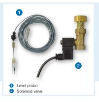
Application For monitoring rainwater tanks for sufficient water level. The backup controller RENA, consisting of control unit RENA, probe and solenoid valve, is designed for fully automatic supply of drinking water to rainwater tanks with connected water station. Continuous operation without frequent on and off cycles, two selectable program times for normal or increased water consumption, with leak monitoring, dry run protection and protection against deposits.
