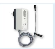
Application For the detection of oil in drip pans below oil-consuming systems, oil pumps, pumping or control stations. Suitable for the following media: water, fuel oil, diesel fuel, motor oils, machine oils, hydraulic oils and similar liquids with a flash point of > 55 °C.
