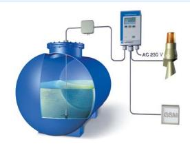
Monitoring of the level in an outdoor rain water tank. A combined alarm light and horn is connected in the vicinity of the tank; TankControl 10 is installed inside the building. It is also possible to connect a float switch to monitor for backflow from the drain. The system can be extended by a GSM-based event reporting system.
