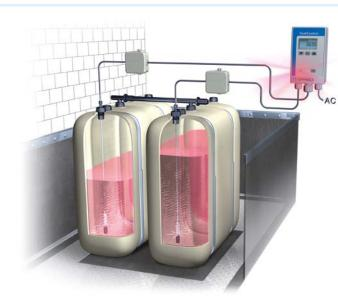
Monitoring of the levels in two communicating tanks. A submersible probe is installed in each tank. If the level difference exceeds a defined value, the unit triggers an alarm. The causes of the uneven levels can be removed prior to filling. Potential damage as a result of different levels in the two tanks is avoided.
