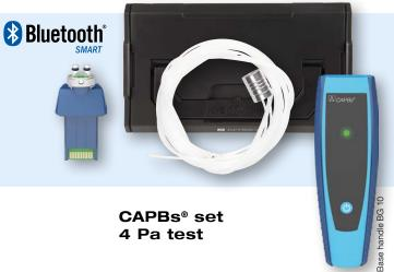
Application If multiple heat systems using indoor intake air and ventilation systems are operated in a closed space, this can result in a hazardous low pressure. The 4 Pa test set, consisting of the sensor module pressure/temperature CAPBs® sens FP 10 with hose kit in the system case S, it is possible to check and document the low pressure limit value of 4 Pa.
