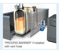
Application For single-line systems with return line in oil fired systems for continuous de-aeration. Suitable for the following media: fuel oil EL (DIN 51603-1) and diesel fuel (EN 590) as well as biofuel and biodiesel with max. 20 % FAME. Also for use in flood hazard areas. The risk of a leak in the return line going unnoticed is removed with Flow-Control. It is no longer necessary to regularly check the return line for leaks.
