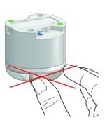
When screwing the sensor head heat alarm AHD into the wireless mounting base ASD 10, hold it at the upper third.
